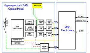
Fig. 4 – PRISMA Instrument block diagram
