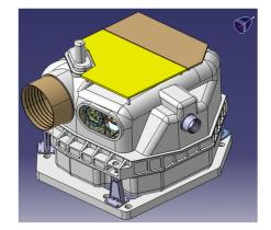
Fig. 5 – Hyperspectral / PAN Optical Head layout
